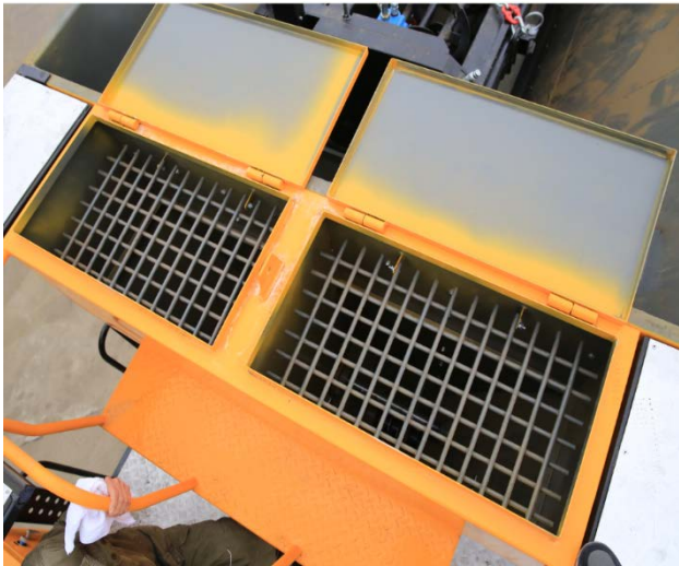
2 mineral fillers tank
