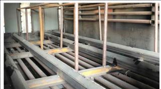
Heating transfer oil pipeline is fully covered under the track, on both sides of the wall and the bottom of the equipment, Maximizes the heat transfer efficiency.
