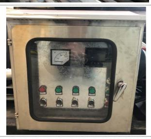
Temperature control panel. Heating transfer oil temperature can automatically adjust by set temperature which can sale the fuel.
