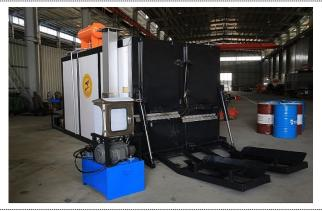
Hydraulic drum-loading system with electric motor driven hydraulic power unit. the front door also controls by hydraulic cylinder to enhance the sealing.
